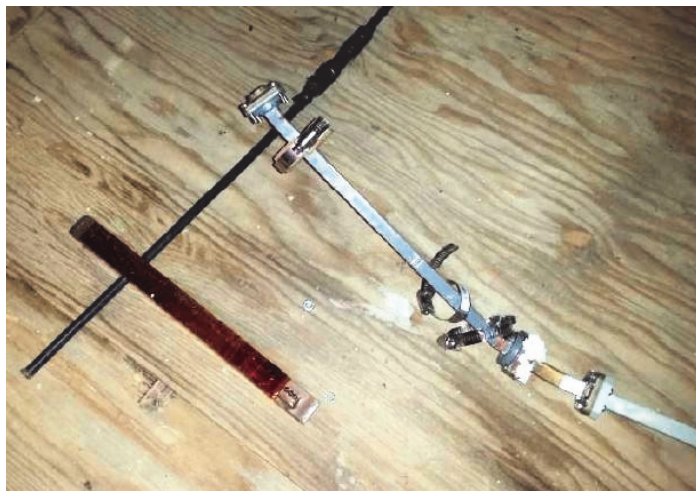
Bent waveguide with slot antenna ripped out of flange
